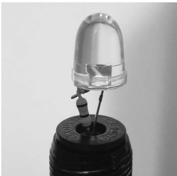
Figure 9. Red LED with voltage dropping resistor plugged into a Mini Maglite flashlight.
