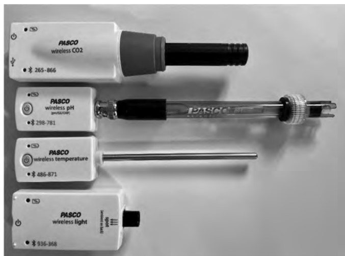
Figure 3. Wireless sensors used. From top to bottom: wireless CO 2 sensor, wireless pH sensor, wireless temperature sensor, and wireless light sensor from PASCO.
