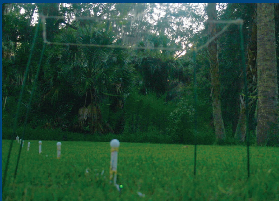
Figure 5. Photo showing the 60 cm x 60 cm box constructed around an artificial female positioned between two light sensors. The small point-source of light appearing in the middle of the four bamboo stakes is the artificial female.
