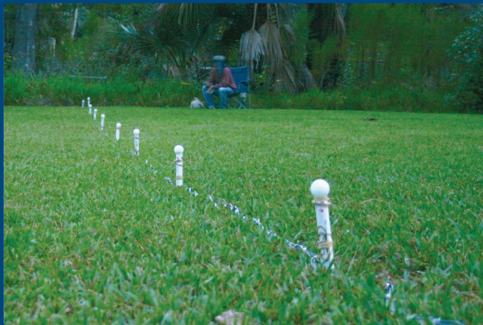
Figure 4. How the nine-light sensor transect is set up at the study site. (Photograph taken at a position near the Plexiglas plate end of the transect.)
