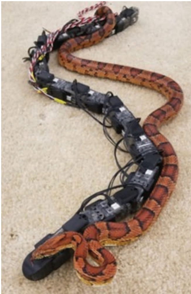
Figure 3. Bio-inspired snake robot developed by Dr. Henry Astley, University of Akron. The robot snake accurately mimics the movements of the corn snake ( Pantherophis guttatus ), also shown in photo. Photo credit: Dr. Henry Astley (used by permission).
