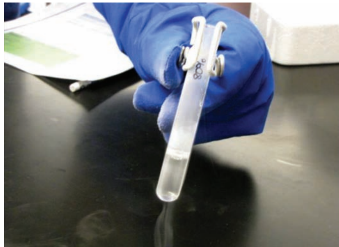
Figure 5. Test tube with 80% glycerol (20% water). Notice that the vitrified solid layer is as clear as glass and there is no ice present.
